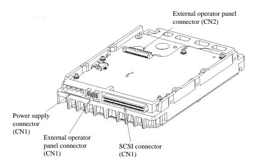
Figure 4.13 Connectors and terminals location (MP model)
